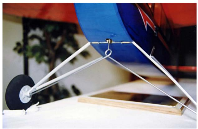
Check out the clever spring landing gear on Tom Pratt's Miss America. That's just a tension coil spring running up inside the fuselage. As the main gear legs splay outward, the spring works against the action to limit wheel spread and bounce. As long as you have all those draggy wires, you might as well have them do something useful.
